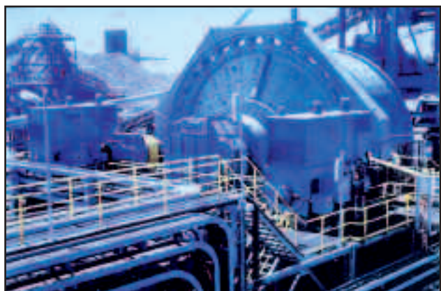
Two PM 600 Couplings on a nickel grinding mill at Leinster in Western Australia.
