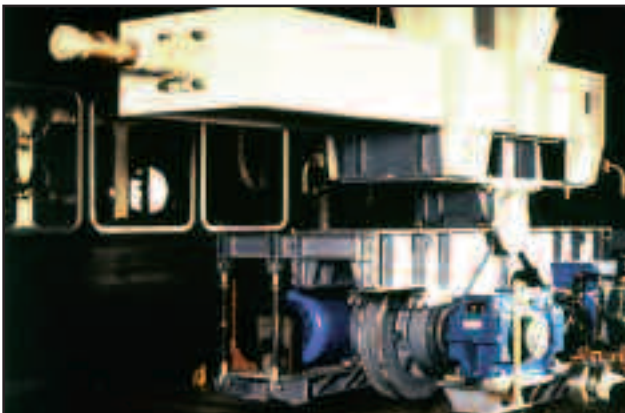
PM 0.7 brake drum coupling and a PM 0.7 spacer coupling on a John Henderson coal charging car at CORUS Dawes Lane.
