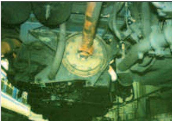
Rail traction. Coupling fitted between diesel engine and transmission via a universal joint shaft.
