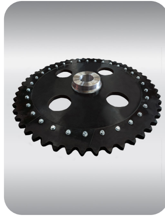
1.75m diameter sprocket with 8 bolted teeth segments to facilitate teeth replacement
