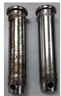
Wear on loaded side of pin
