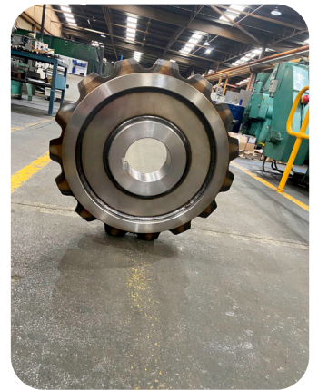
0.8m diameter sprocket with sideplate supports for WH150 chain
