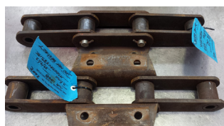
Chain samples with light surface corrosion
